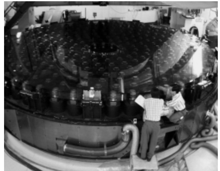
Fig. 6. The polished 8.2m primary mirror at final acceptance test. The invar sleeves attached at the pockets drilled in the back surface for placing the actuators are visible through the transparent glass.
